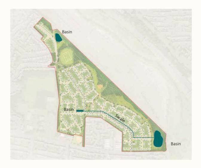
Surface water run-off generated by the development can discharge to the public drainage system.
